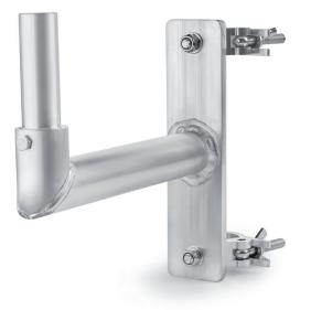
The Speaker Mount d50 from MILOS features a 35mm spigot that fits standard speaker holes and has an SWL of 70 kg. Its can be positioned anywhere on vertical 48 – 50mm truss tubes via two clamps positioned on the rear of the mounting assembly.
